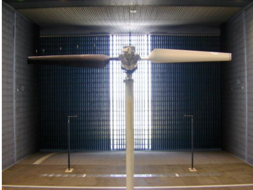
Figure B.1: Photograph of the UAE Phase VI test turbine in the NASA/Ames wind tunnel
